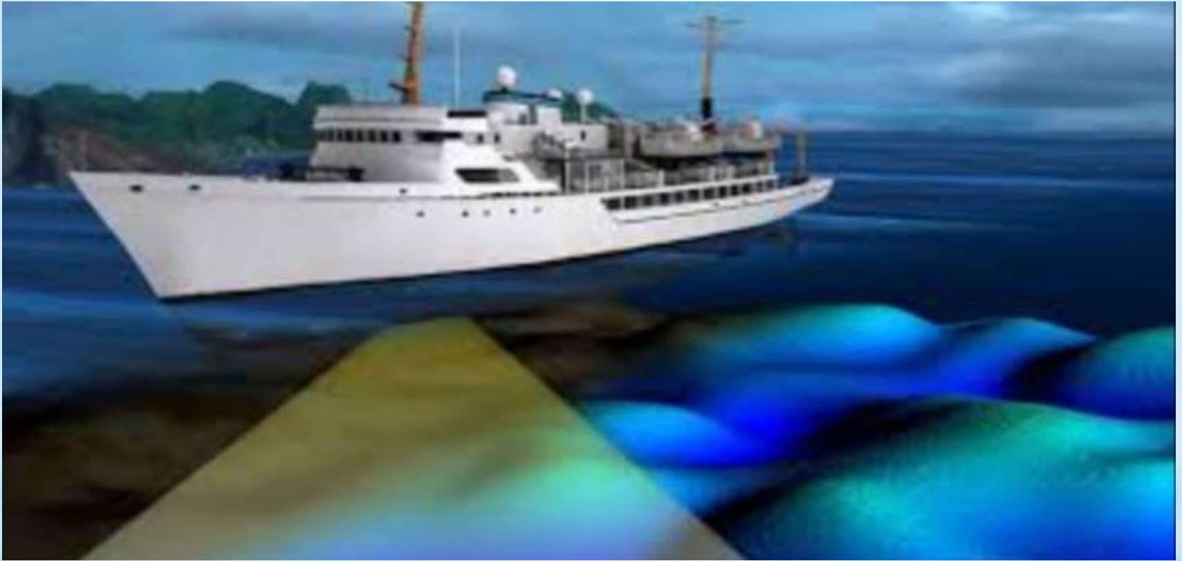
Fig 3: A simulated image showing the multi beam Echo Sounder. Source: Ocean News and Technology Magazine(2019)
